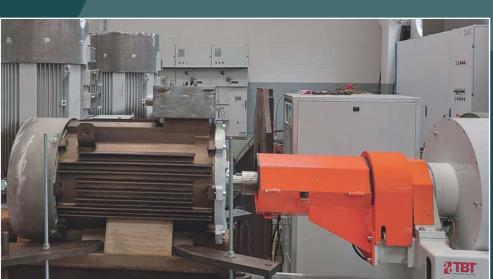
Test bench industry 4.0: load test on marine motor
