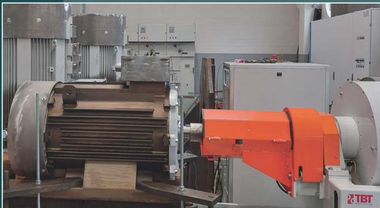
Test bench industry 4.0: load test on marine motor
